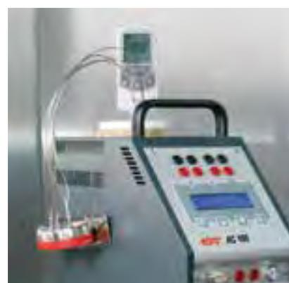
Precision measurement and testing equipment such as thermometers and data loggers should be checked and calibrated regularly.
